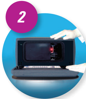
2 Place FastPack® into the FastPack® IP Instrument
