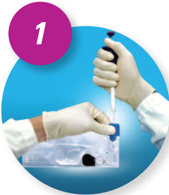
1 Dispense sample into the FastPack® Injection Port
